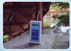
Particle test in **Canada** outdoors (Particle Level: **4,604** particles/litre).
