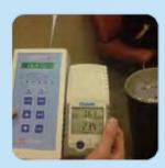
Particle level in a smoking area: More than 1,600,000 particles/litre. (l.e. 27 times higher than AQG.s).\*
